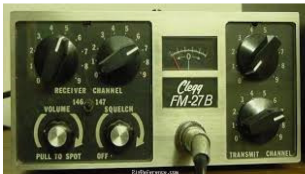
The Clegg-27B 2 meter transceiver that the author still uses today with his homebrew sub-audible tone generator.
